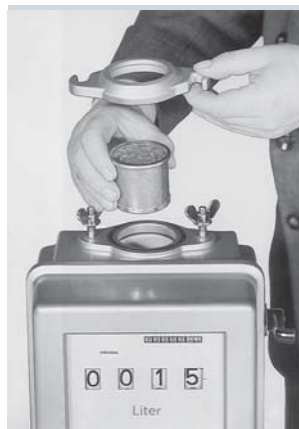
Quantity preset register with desiccant cartridge removed
